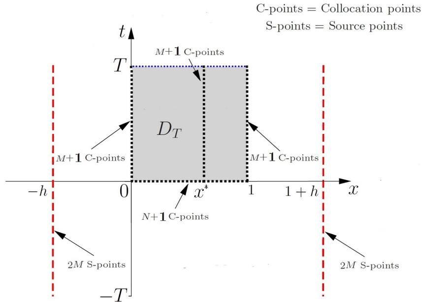
FIGURE 1. The representation of the placement of source and collocation points.
