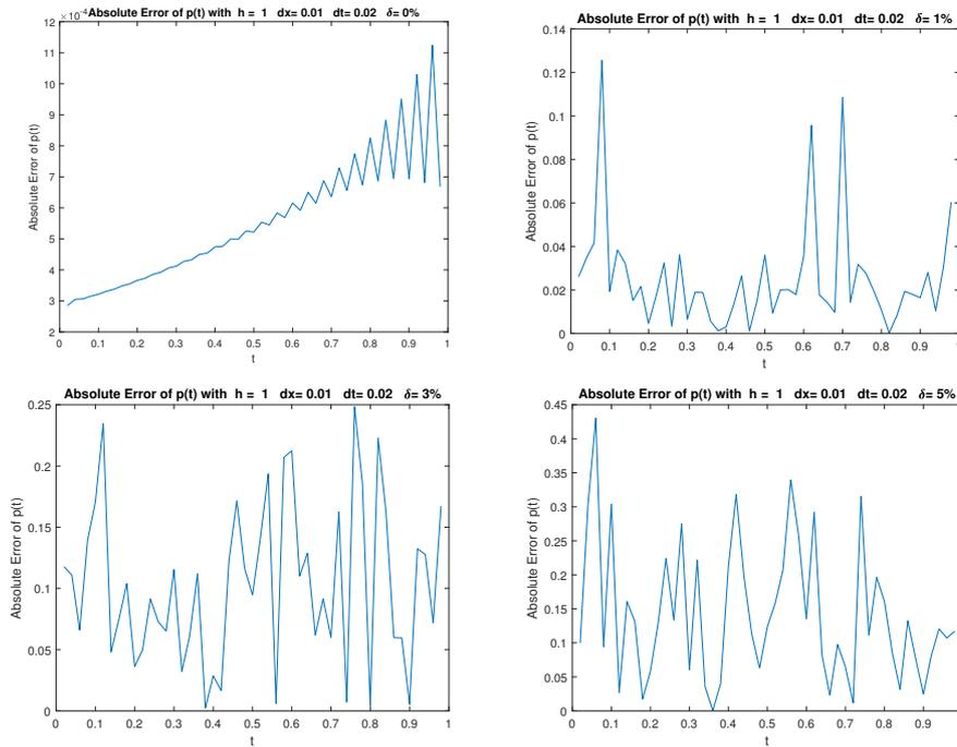
FIGURE 2. The absolute error of the numerical solution of  $p(t)$  for different values of noise level  $\delta$  with  $M = 50, N = 100, h = 1$  for example 1.
