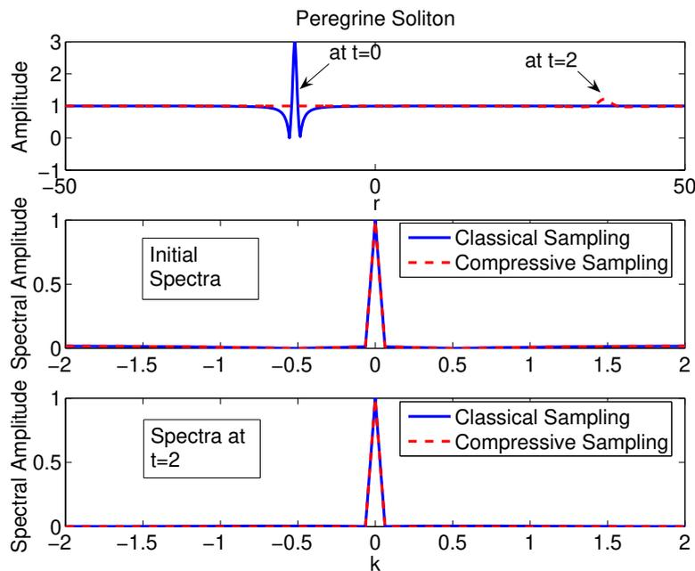
FIGURE 1. a) Peregrine soliton at  $t = 0$  and  $t = 2$  b) the Fourier spectrum of the Peregrine soliton at  $t = 0$  obtained by  $N = 1024$  classical and  $M = 64$  compressive samples c) the Fourier spectrum of the Peregrine soliton at  $t = 2$  obtained by  $N = 1024$  classical and  $M = 64$  compressive samples
